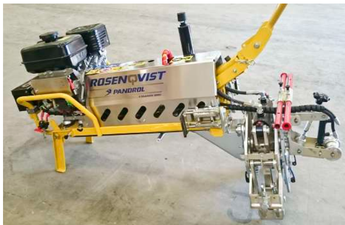
Fig. 20: Parked off track (FC/FE work head)
