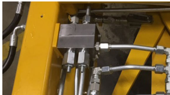
Fig 20. Spread retraction pressure adjustment
