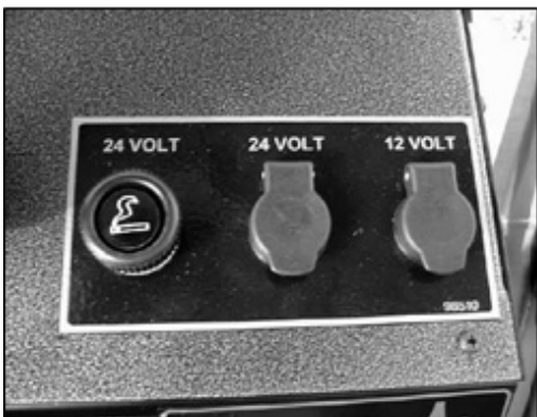
Fig 6. Examples of charger plug connector in driver's cabin
