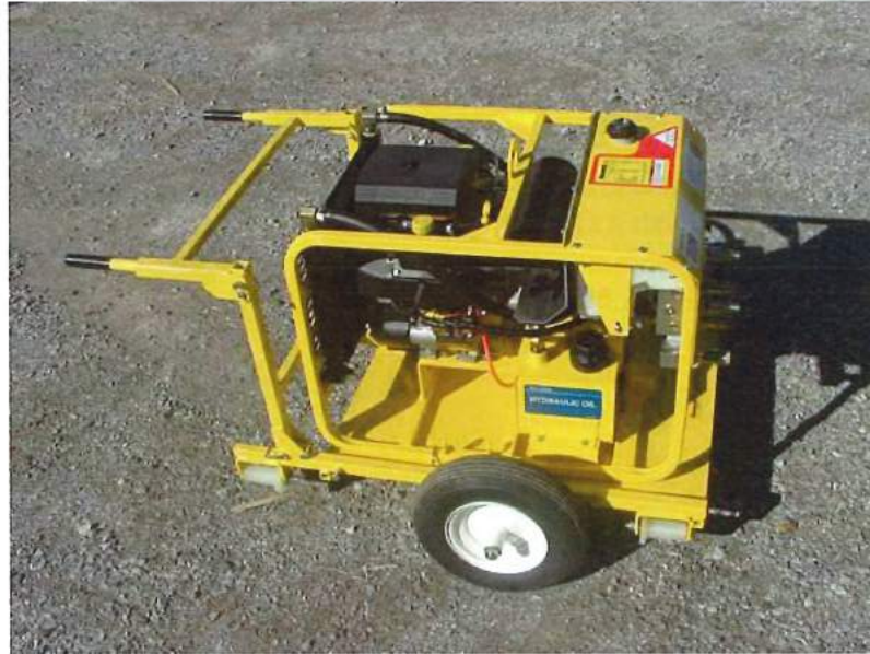
Shown above with Pandrol 00100K power unit (off track mobility)
